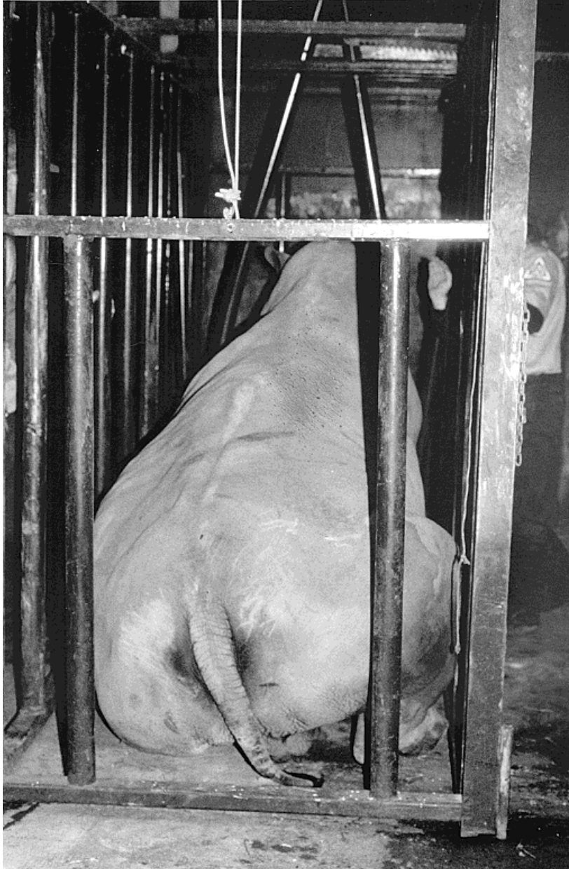
Fig. 3. Chute 3. A wide, operable space in the guillotine gate is needed with this wide chute.
