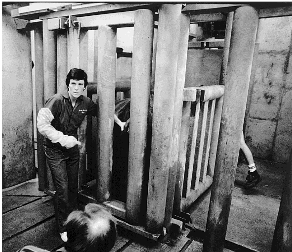
Fig. 1. Chute 1. Large bars in the rear gate pin the operator when animals move side to side.
