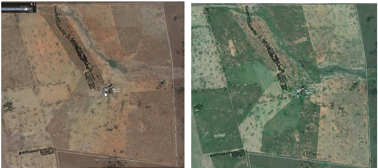
Figure 8: May 2017 Google Earth scene at BDR (left image) and March 2018 image (Right image), each showing Camps 1/ 2 (two at top right), 3 /4, (two at bottom right), 5/6 (top left) and HF (bottom left), with lighter, grazed camp-sections and darker, resting sections switching sides between the 2 images.
