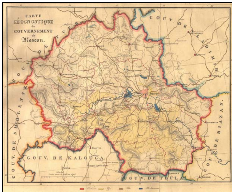
Figure 6. Fischer’s geognostic map of the Province of Moscow from Oryctographie (1830–1837). Red = Limestone; Yellow = Gypsum; Darker yellow (now faded and indistinct) = Sandstone; Blue = Ferruginous alluvium.
