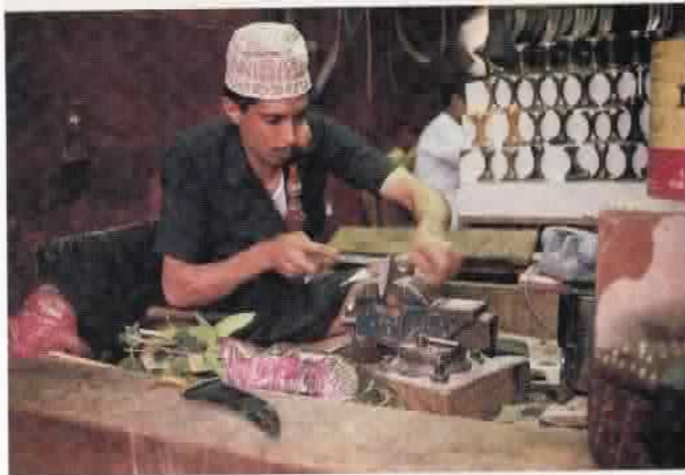
A dagger-maker in the Yemeni souk, or marketplace, uses a file to shape a rhino-horn handle. He can make 20 hilts from one horn. Because rhinos are so rare, the price of such a dagger starts at $1,500.
