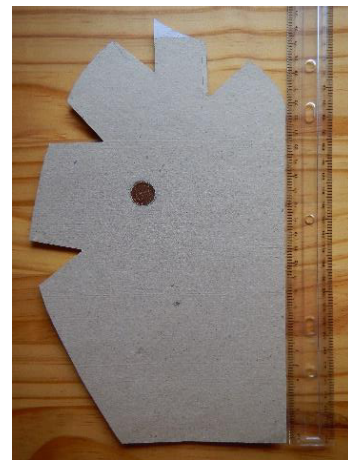
Figure 10 The template used to guarantee that every notch is identically positioned on the dummy rhino ear. The hole notch is congruent with a ZAR 10 cent coin.
