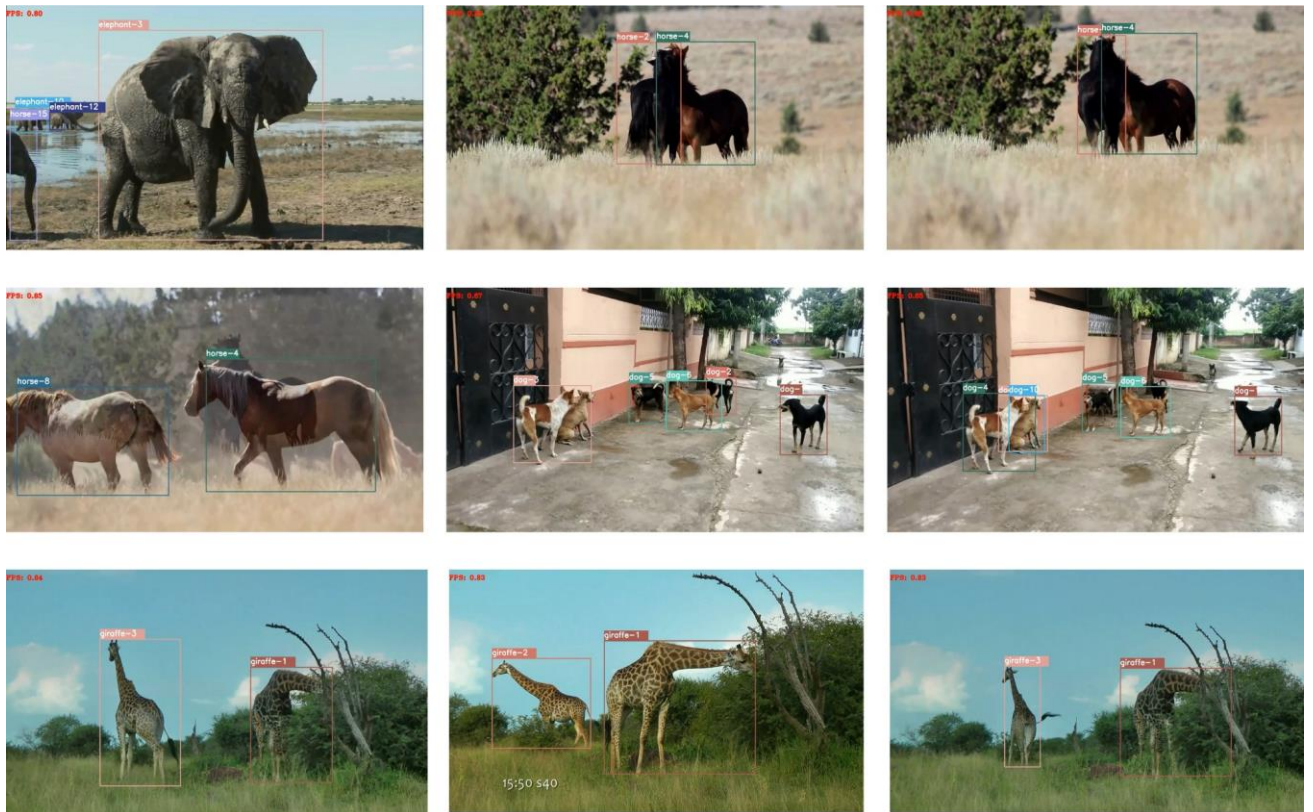
Figure 3. Result samples from animal motion tracking using YOLOv4 and Deep SORT
