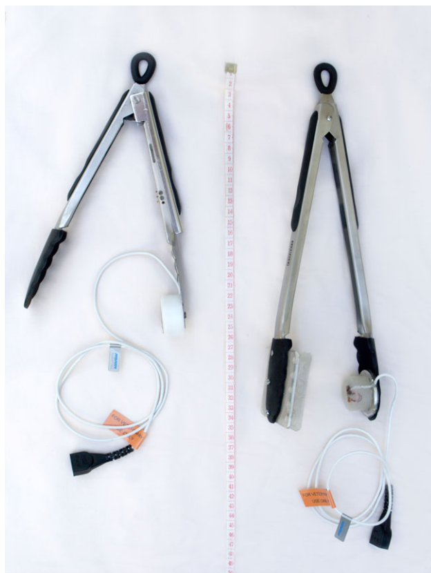
Fig 1: Comparison of the two pulse oximetry sensor prototypes N1 (left) and N2b (right) for buccal reflectance pulse oximetry in horses: general view. Please note the difference in the length of the tongs (prototype N1: 23 cm, prototype N2a and N2b: 31 cm).
