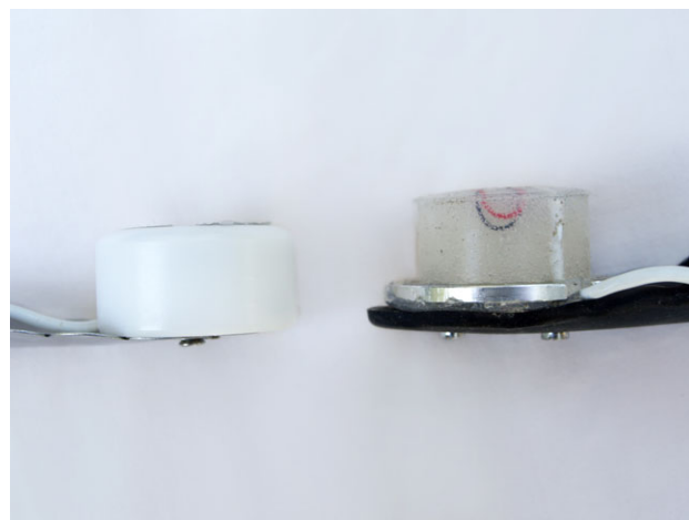
Fig 2: Comparison of the two pulse oximetry sensor prototypes N1 (left) and N2b (right) for buccal reflectance pulse oximetry in horses: close-up view of the sensor heads. Please note the different distance between sender and receiver (prototype N1 and N2b: 13 mm, prototype N2b: 10 mm), the shape of the silicon bedding towards the mucosa (plane in prototype N1 and N2b, convex in prototype N2b) and presence of the surrounding plastic from the original sensor (present in prototype N1, removed in prototype N2a and N2b).
