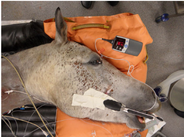
Fig 3: Pulse oximetry sensor prototype N1 for buccal pulse oximetry in horses in place.
