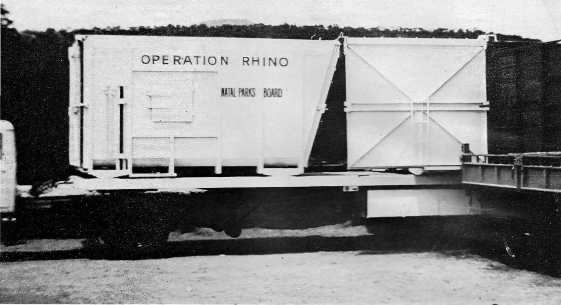
Plate 17 Swivel crates for rhinoceros long-distance transportation: the sloping front exit door prevents damage to horn. Each crate holds two rhinoceros and has a passage for attendant.
