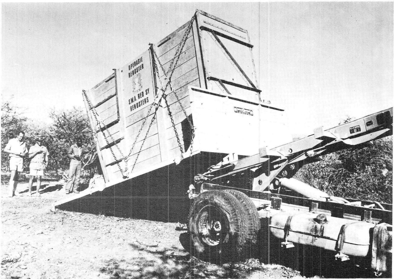
Plate 2. The multilift system used for loading black rhinos.
