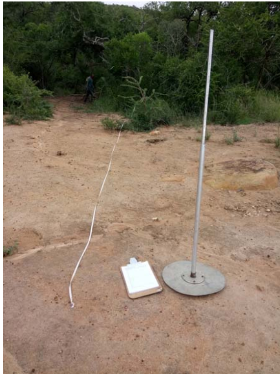
Figure 2. The DPM (disc pasture meter) consist of a metal pole with a movable disc. It measures the grass biomass under the disc that is dropped from the top to it reached the grass.
