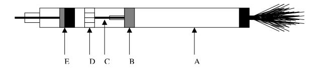
**Figure 2.** The air has pushed plunger (E) forward moving the pin into the needle and expulsing implant (F) depositing it in the subcutaneous tissue.
