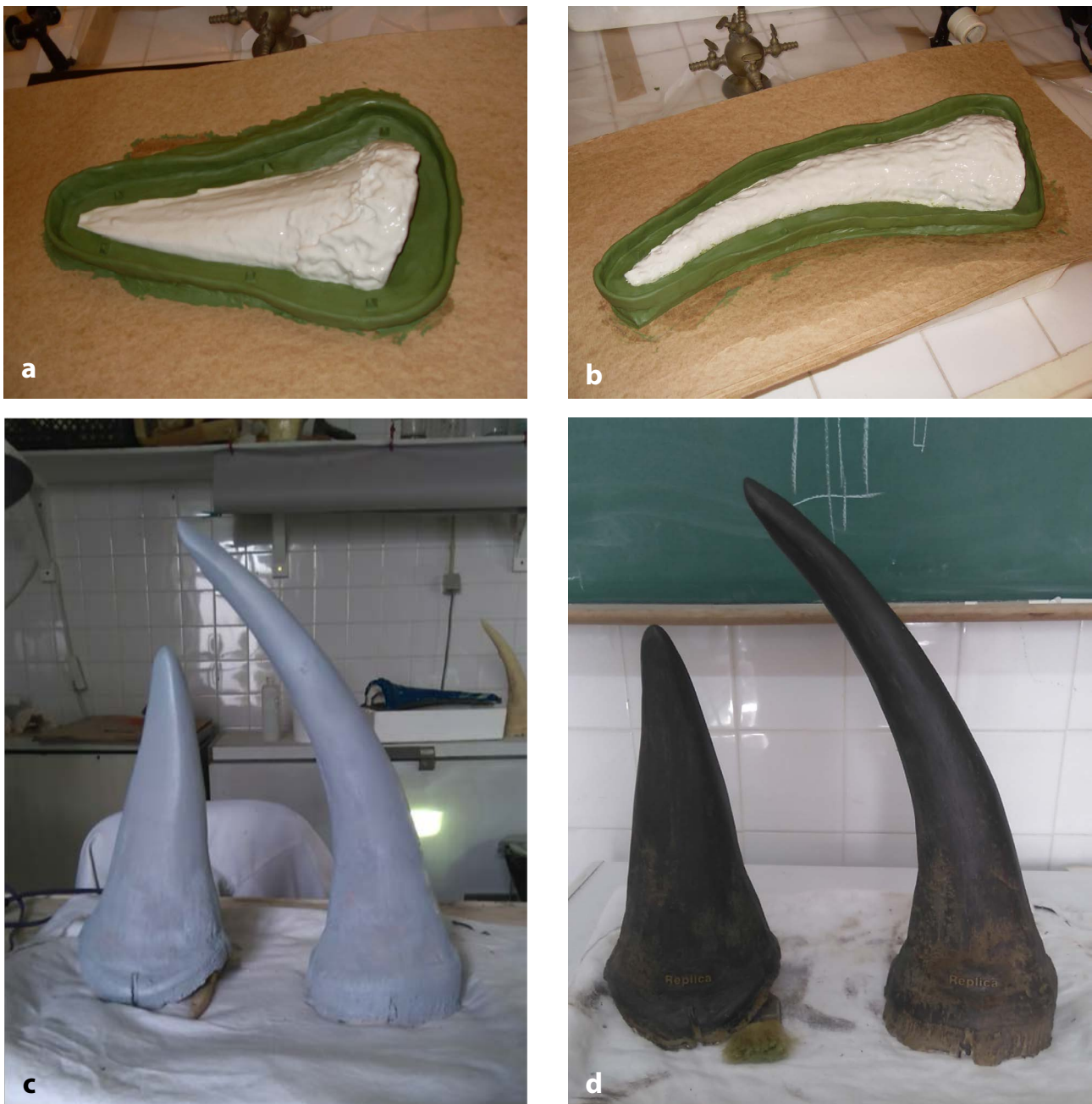
Figure 10. Details of the moulds, support moulds and finished horn replicas created by Pedro Andrade (MUHNAC).
