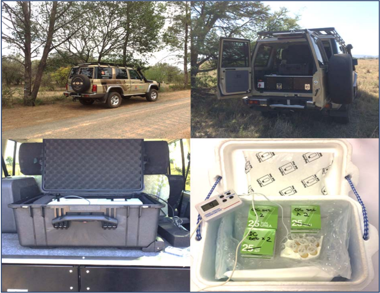
Figure 4: The field performance study. Clockwise from top left: the 4x4 vehicle out in the field; the VetTest placed in the back of the vehicle; VetTest slides and QCM stored in a polystyrene box on ice; the VetTest protected by a hard moulded plastic box.
