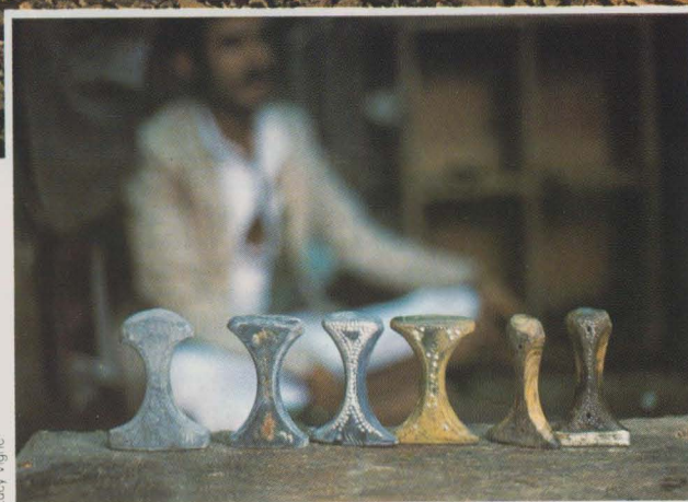
This is a set of dagger handles, showing the six different stages of handle-making.
