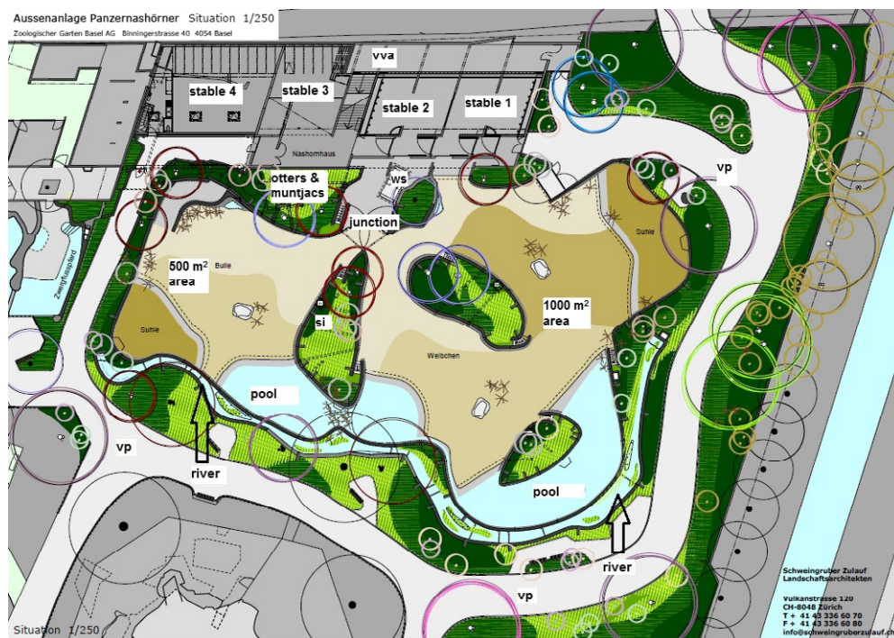
Fig. 2. Site plan of the new Greater one-horned rhinoceros Rhinoceros unicornis enclosure at Zoo Basel, Switzerland: si. separating island (80 m 2 ); vp. visitor pathway; vva. indoor visitor-viewing area; ws. weighing scales. Access to the outdoor area from the stable 1 is directly into the 1000 m 2 outdoor enclosure to the right, while from stable 2 access is via the junction area, past the weighing scales and into the smaller 500 m 2 outdoor area to the left. The stables for Asian small-clawed otters Amblonyx cinereus and Chinese muntjacs Muntiacus reevesi are indicated. Zoo Basel.
