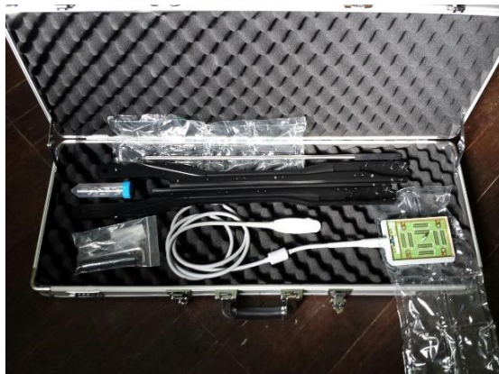
Plate 23. The complete set of OPU probes and CX 11 probe
