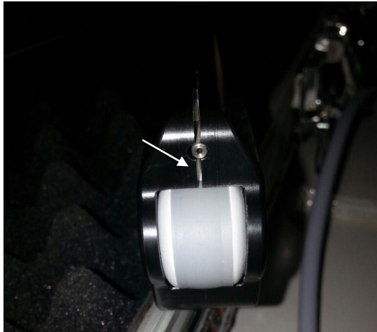
Plate 22. The gap (arrow) is seen when the transducer is placed together with the needle
