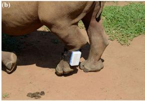
**Fig. 2** Biotelemetry collars. **a** Fitted around the necks of four sheep. The accelerometer *x*, *y* and *z* axes are associated with left–right, up–down and forward–backward movements of the sheep, respectively, **b** fitted around the black leg of a rhinoceros. The accelerometer *x*, *y* and *z* axes are associated with the up–down, forward–backward and left–right movements, respectively
