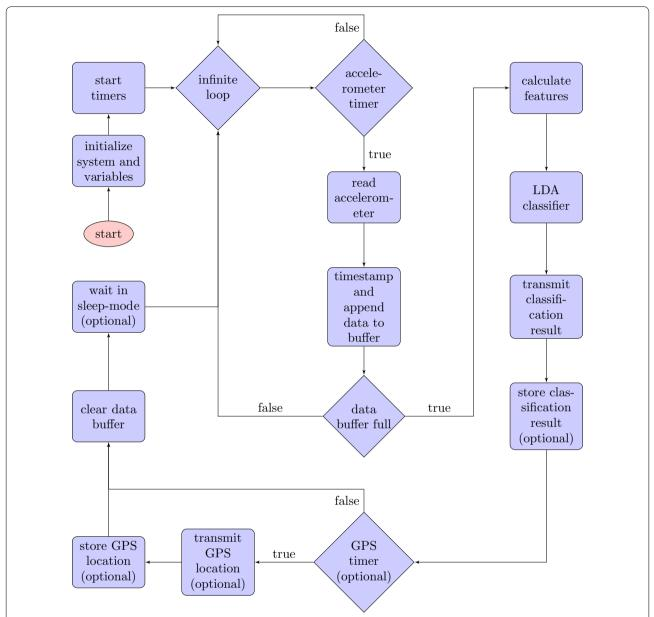
**Fig. 5** Software flow diagram of the animal-borne behaviour classification system. Accelerometer sampling is controlled by a timer to ensure a constant sampling frequencies of 100 Hz for sheep and 40 Hz for rhinoceros. The GPS acquisition interval is determined by a second timer
