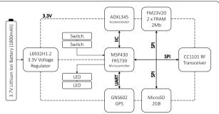
**Fig. 1** Block diagram of the hardware design of the biotelemetry tags. A MSP430 ultra-low-power microcontroller communicates with the accelerometer using I<sup>2</sup>C, the GPS using UART and the FRAM, MicroSD card and RF transceiver using SPI. Two tactile switches and two light-emitting diodes were included for software functionality selection and indication purposes, respectively
