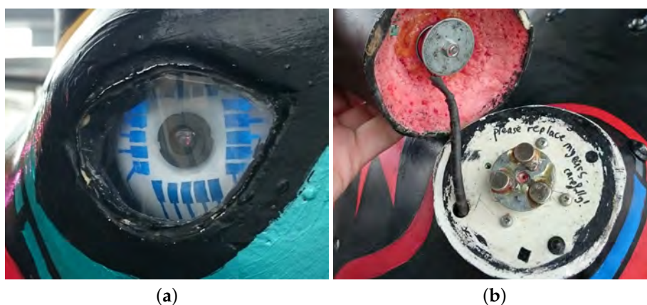
Figure 4. (a) detail of Erica's eye assembly; (b) detail of Erica's detachable ears.
