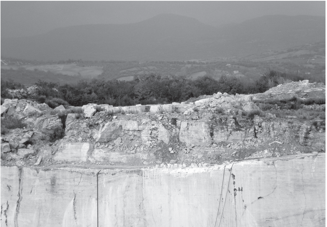
Fig. 2. Saturnia quarry from Montemerano-Manciano at present days. a) arenaceous level with decomposing travertine blocks; b) travertine compact level.
