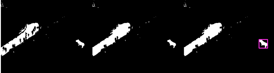
Figure 3.2.2: Left: Original, Middle: Original after morphological operations, Right: Same as the middle with bounding boxes with area constraints
