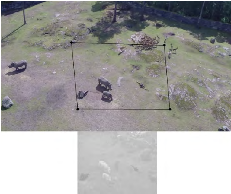
Figure 3.1.1: The black box in the upper image shows how the lower, thermal, image fits the RGB image. Note that the thermal (lower) image is scaled by a factor 2 compared to the RGB image
