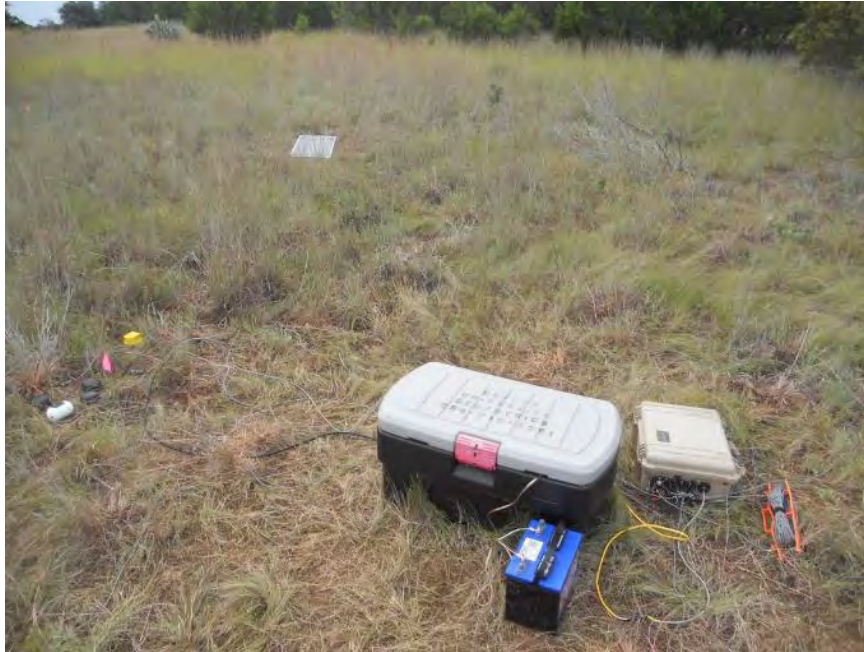
Figure 24. Setting up the RefTek site.
