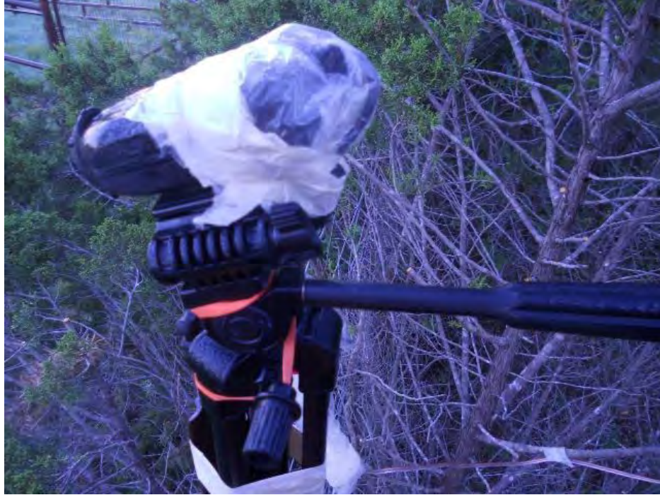
Figure 21. The waterproofed Drift video camera.
