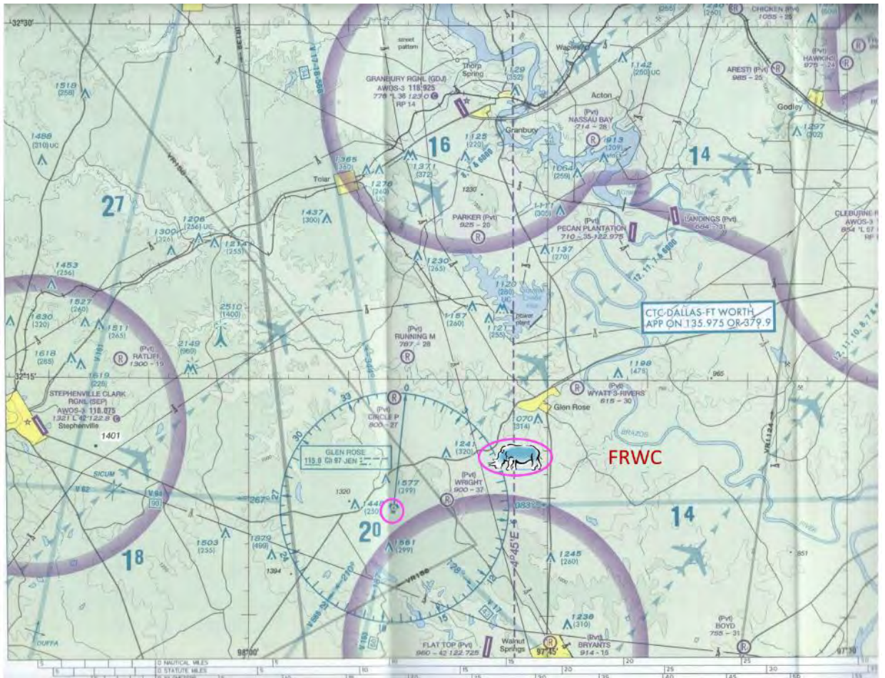
Figure 27. DFW terminal area chart. Glen Rose VOR is the center of the compass rose (shown in pink) instructing aircraft planning to land in the metroplex from the southwest, to fly along the dotted line heading northeast past FRWC (at the location of the rhino). Wright private airstrip lies between.
