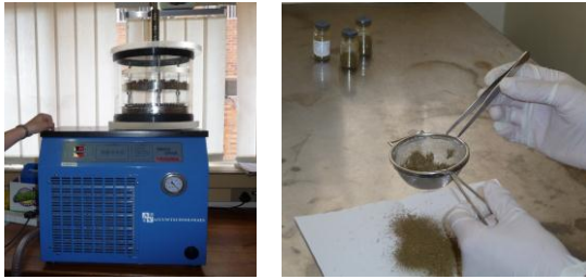
Figure 7. Vacuum oven (left) and sieving the dry samples (right).
