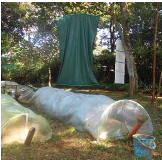
Biogas digester units
