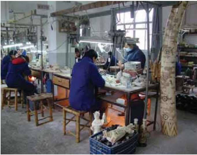
Factory workers carve ivory from both mammoths and elephants and also make large bone items such as the giant tusk on the right consisting of wood covered with tile-like carved pieces of cow bone.
