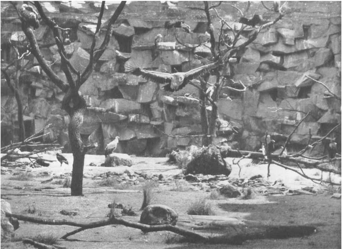
53. top. View of the new birds of prey aviary at East Berlin Zoo. The aviary measures 60 m long, 8 to 27 m wide and 9 m high, covering a ground surface of about 1,200 sq. m (see pp. 69-70). All supports are outside the aviary, thus giving the birds maximum flying room. The aviary is backed with large grey blocks of Lausitz granite freestone and behind there are winter quarters for non-hardy birds of prey. It contains about 50 birds of prey belonging to 13 species. Werner Engle E. Berlin
