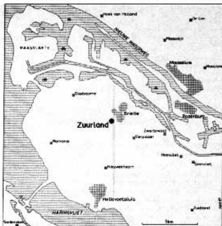
Fig. 1. Map showing the location of the Maasvlakte area, borehole Zuurland, and the places (*) where the sediments used for the creation of the Maasvlakte were obtained by suction dredging.
