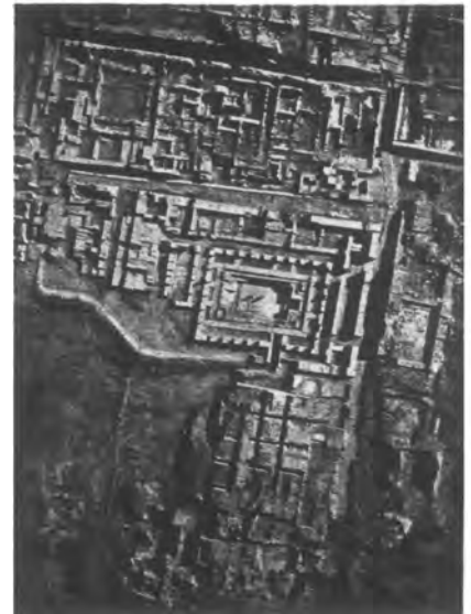
Figure 5 A number of aerial photographs of the site were taken from a hot-air balloon. This was the main technique used in making the photogrammetric survey of the city's architecture. This photograph of the 'Great Bath' was taken from a height of about 100 m. The north-south/east-west alignment of the architecture is clearly discernible. The streets which originally surrounded the building would have enabled processions to walk round it. (Photo: Research Project Mohenjo-Daro).
