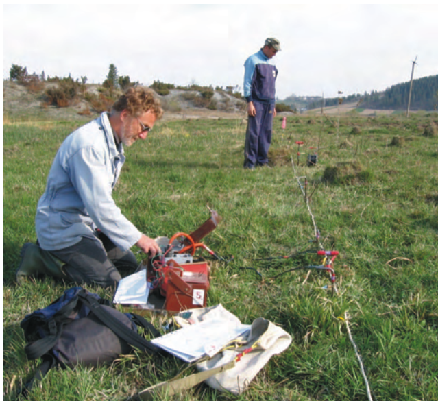
Fig. 13. DC resistivity soundings headed by W. J. Mościcki. Photo by M. Dzieńiewicz
